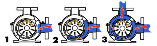
The impeller is withstood eccentrically in a rotating chamber. The rotor retracts the vanes on one side of the body.
