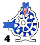
Fluid enters between the gears or through the external ring;
