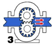
As the gears leave the overlapping area a volume of oil is created and expands on the inlet port.
